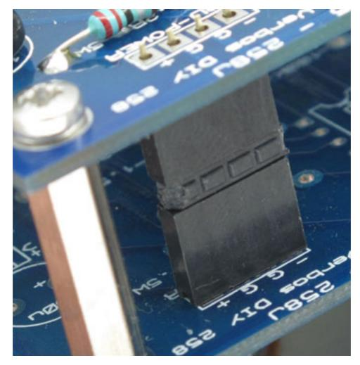
This construction allows the boards to be separated simply
