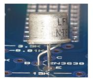
The image to the left shows you how you should insert the transistor once the middle 'B' pin is bent back.
