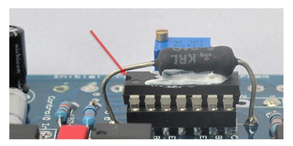
Wipe away any excess paste, make sure it's only on the top of the IC and the underside of the tempco. You really do only need a very small amount to make contact where the cylindrical body of the tempco meets the top of the IC.
