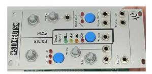
Hand tighten all the nuts and make sure the switches are sitting square and that the switch caps are not rubbing against the panel.
