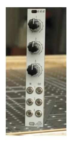
On a modular synthesizer, attenuators are an important building block in pretty much every part of your patch for both CV and audio duties.
