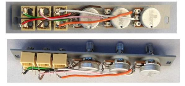
23 – The final task is fitting the knobs. Turn all the pots fully counter-clockwise or fully OFF.
