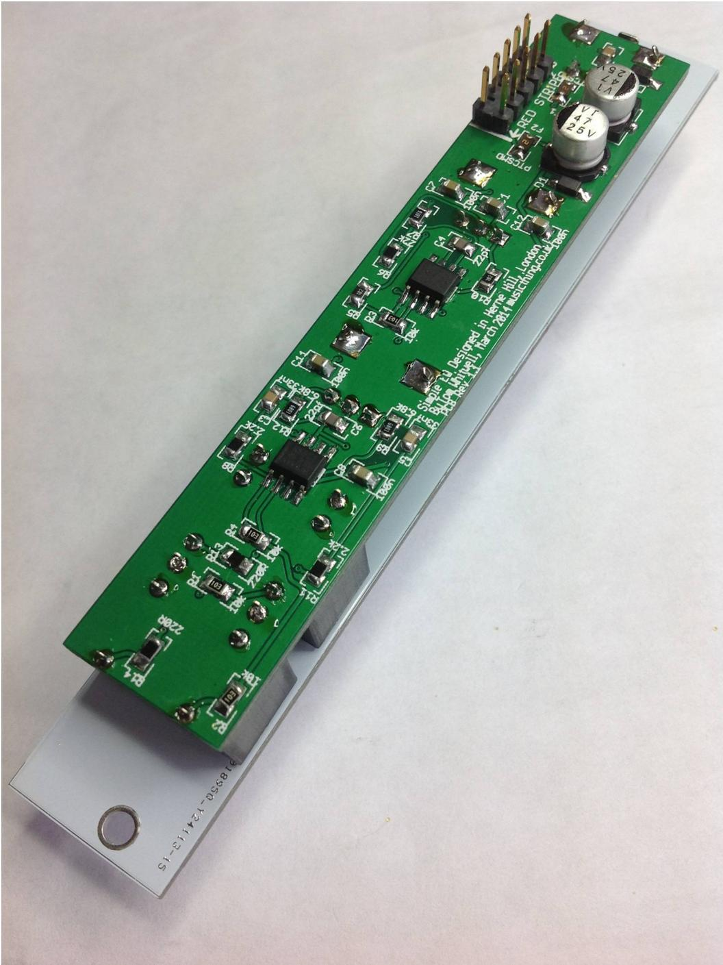
And thats the soldering done. All you need to do now is tighten up the nuts on the jacks and on the pots, then fit the knobs.
