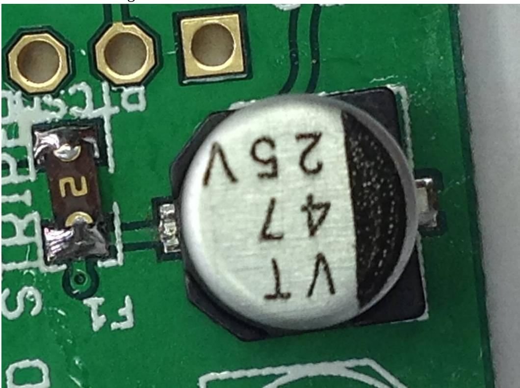
Check the capacitor's sides still sit squarely with the markings on the PCB's silk screen. If the capacitor is miss-aligned, re-apply the soldering iron to the pad & gently twist the capacitor until it's correctly aligned. The pin on the other end of the capacitor should be roughly in the middle of its pad.
