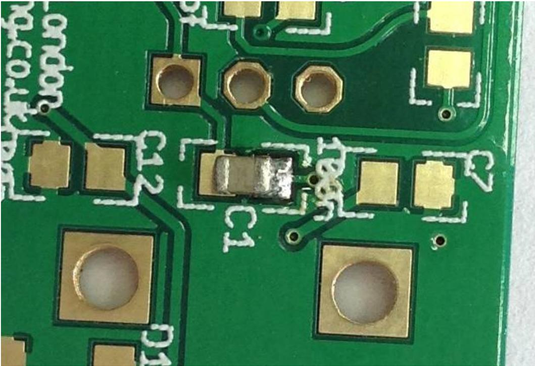
*Illustration 12: ceramic capacitor soldered on one side*
