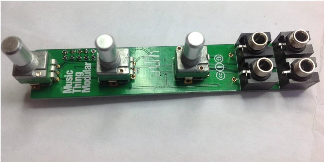
Fit the panel over the pots & jacks, then fit the washers & nuts onto the pots and jacks. Do the nuts up finger tight. The retaining clips on the pots should keep everything in place whilst you do this. The panel should now be parallel to the PCB.
