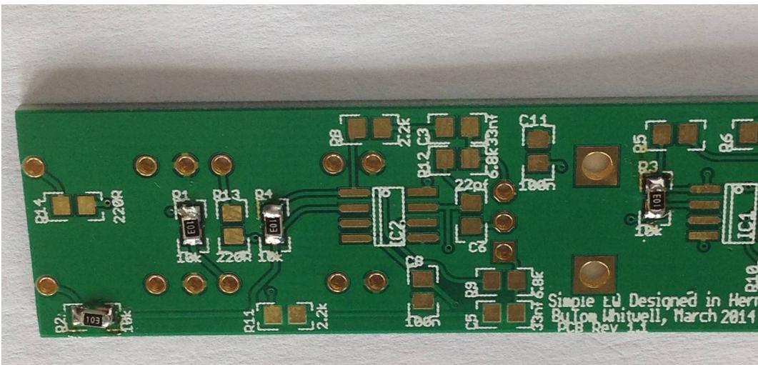
Now install the 2 x 2K2 resistors R8 & R11. Note the one used in the picture here doesn't have the value written on the black side. That's not a problem.
