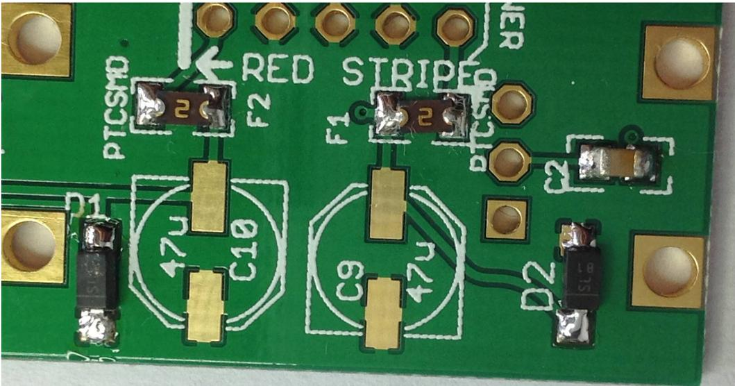
*Illustration 18: Diodes D1 & D2 installed, with line identifying cathode towards the PCB edge*
