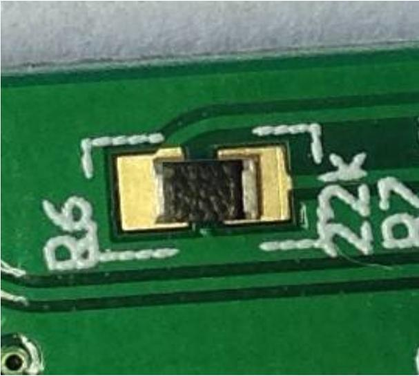
*Illustration 7: SMD resistor located centrally on pads*
