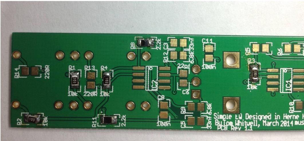
Now install the 2 x 220R resistors R13 & R14:
