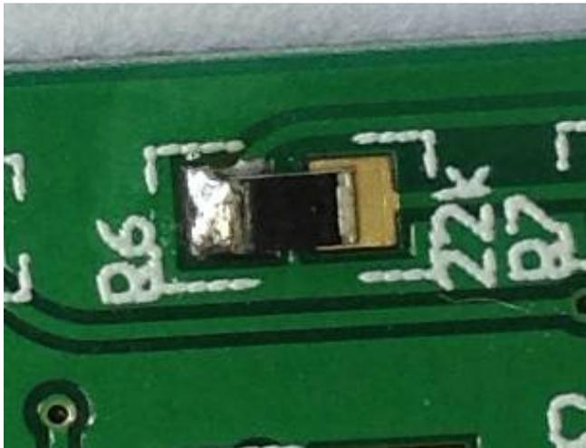
*Illustration 8: resistor soldered to one pad*
