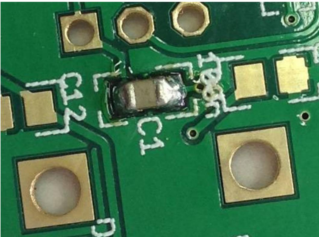
*Illustration 13: ceramic capacitor soldered on both sides*
