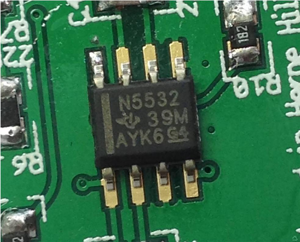
*Illustration 23: NE5532 with one pin soldered*
