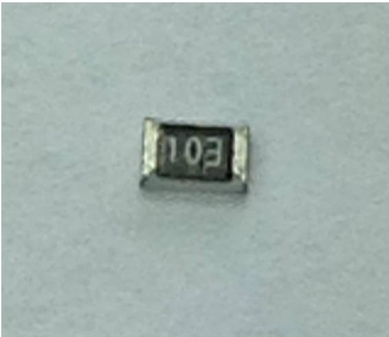
*Illustration 5: 10K SMD resistor top view showing the value "103".*
