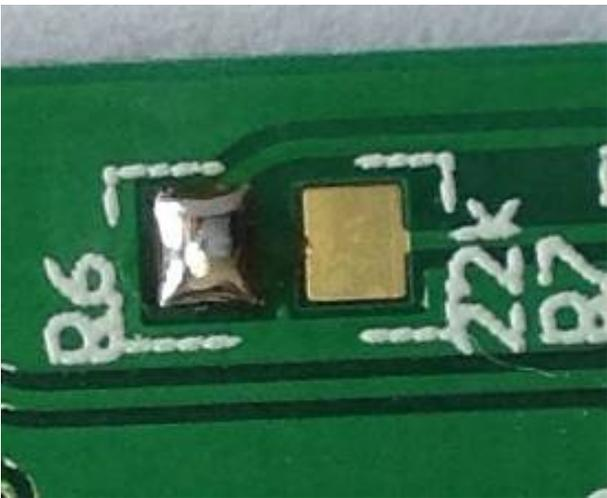
If you think you've applied too much solder to the pad, you can remove this with solder wick. Place the wick on top of the blob of solder, apply the tip of the soldering iron briefly. The wick will soak up the solder. The wick will probably remove almost all the solder so you'll need to re-apply a small amount.
