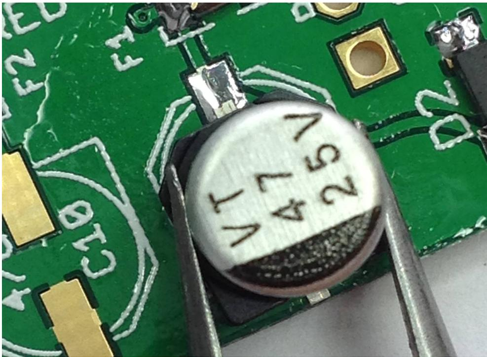
Apply the tip of the soldering iron to the other end of the pad. Once the solder on the pad melts, push the capacitor forward along the pad with the molten solder until its pin comes into contact with the soldering iron tip and the capacitor is now aligned with the silk screen on the PCB. Remove the soldering iron.
