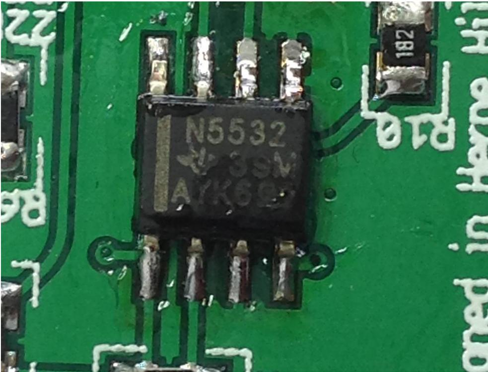
*Illustration 25: NE5532 with all 8 pins soldered. Note the flux covering the pins and the package. This will be removed during cleaning.*
