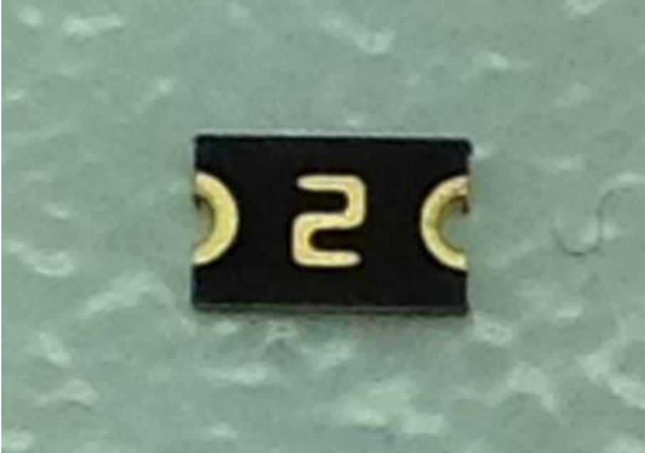
*Illustration 14: PTC fuse top side. Install with this face upwards.*
