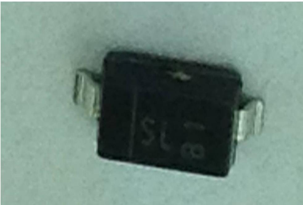
*Illustration 17: Surface mount diode, showing line identifying cathode as the left hand pin*
