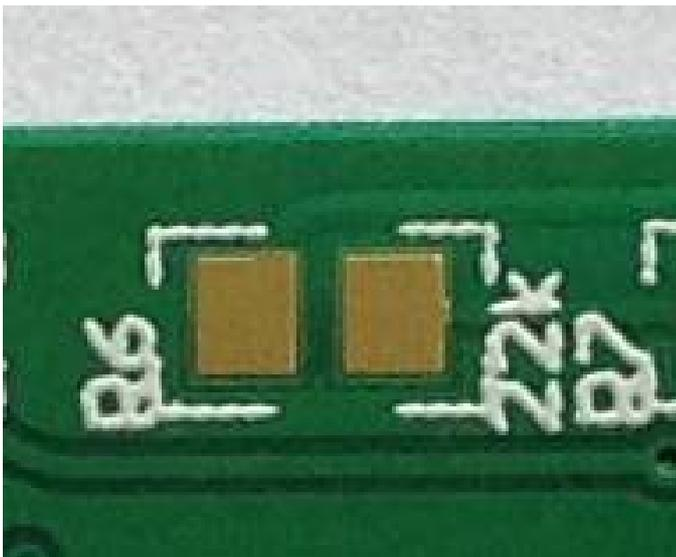
*Illustration 6: SMD resistor pads and silk screen on PCB (showing R6)*
