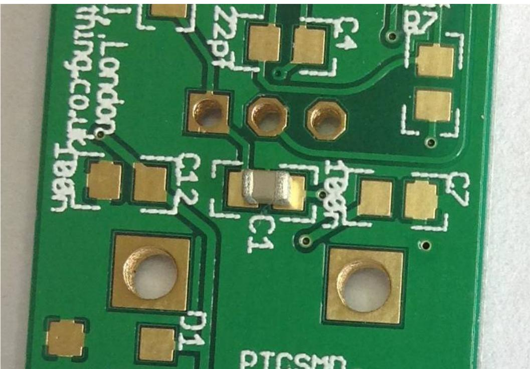
*Illustration 11: ceramic capacitor aligned on PCB pads*
