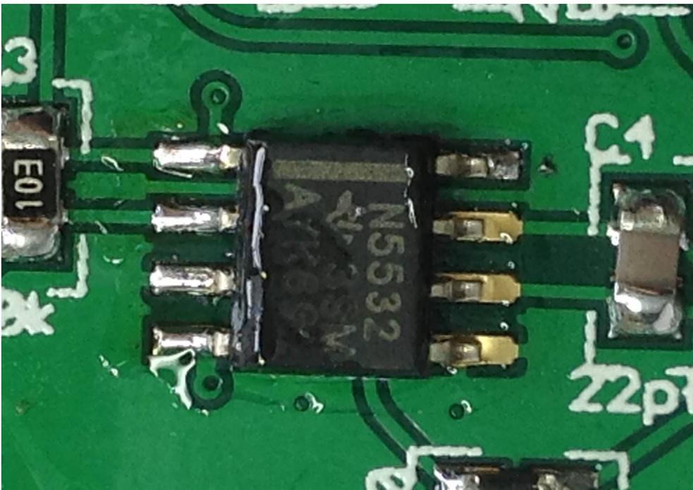
*Illustration 24: NE5532 with 5 pins soldered.*
