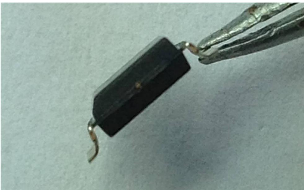
*Illustration 20: Surface mount op-amp showing sloped face on packaging.*
