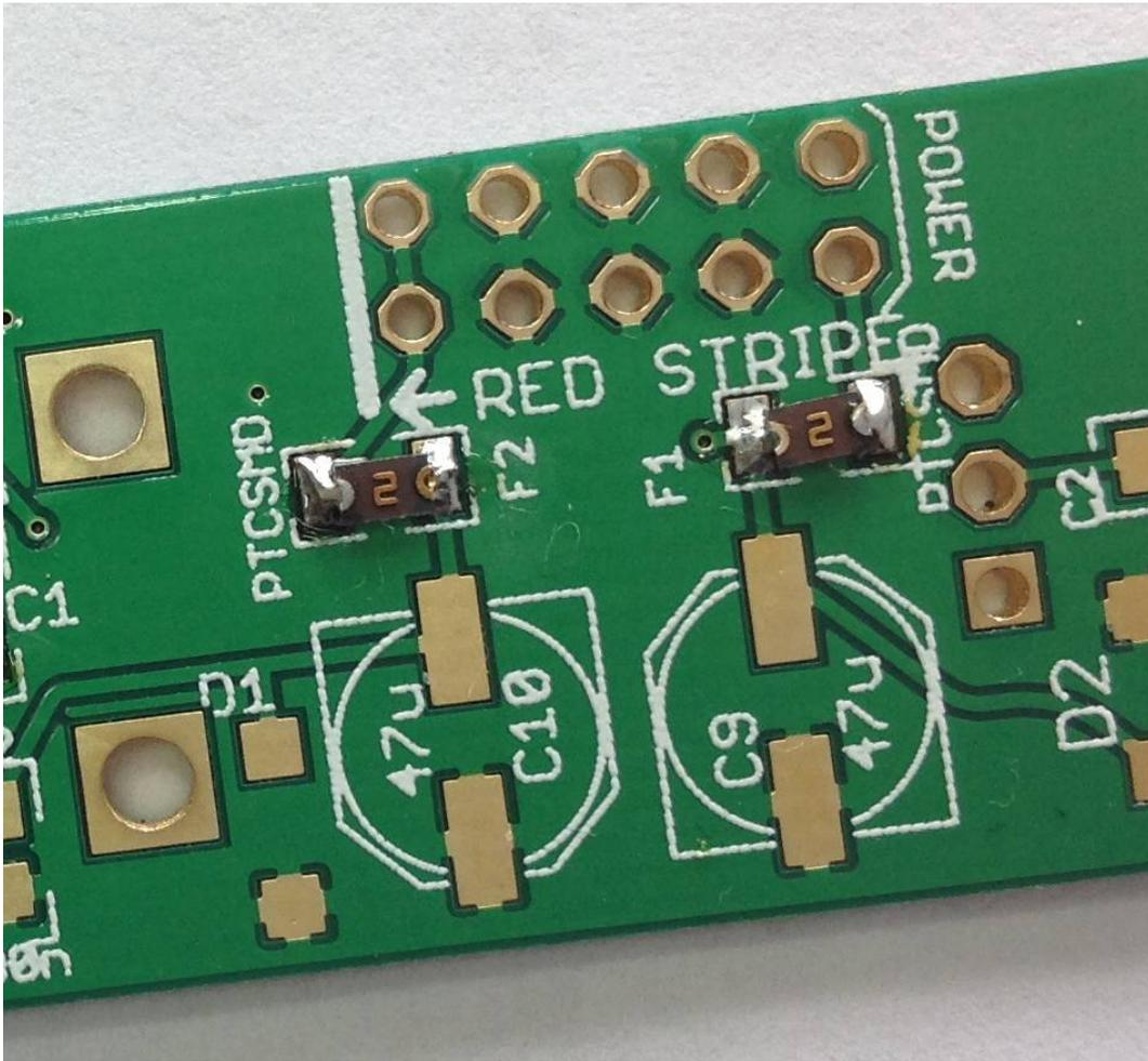
Illustration 16: PTC fuses F1 & F2 installed on the PCB
