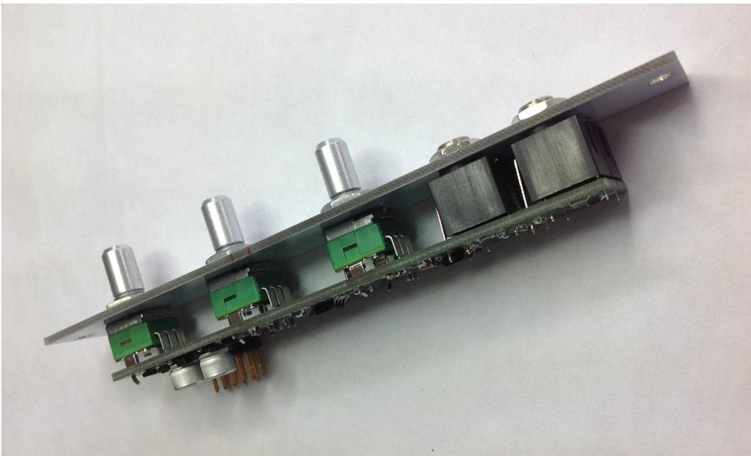
Turn the assembly over so the component side of the PCB is facing upwards. Solder one of the Tilt jack pins nearest the bottom of the PCB. Turn the assembly on it's side & check that the jack is in contact with the PCB. If there's any gap between the jack & the PCB, apply the soldering iron to the pin whilst squeezing the panel & PCB together so that the jack is sat flush to the PCB. Solder the
