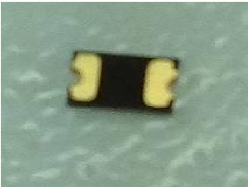
*Illustration 15: PTC fuse bottom side. Install with this side on the PCB.*
