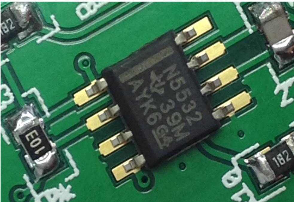
*Illustration 22: NE5532 op-amp located on the pads at IC1 prior to soldering*
