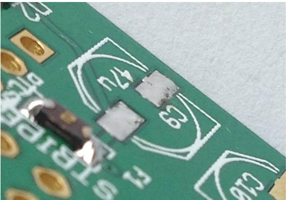
Now, if you're using a flux pen, apply some flux to the PCB pads and also to the capacitor's pins. The flux will help the solder flow into the joint between the pad & the capacitor's leg.
