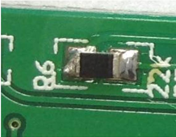
*Illustration 9: resistor soldered to both pads*
