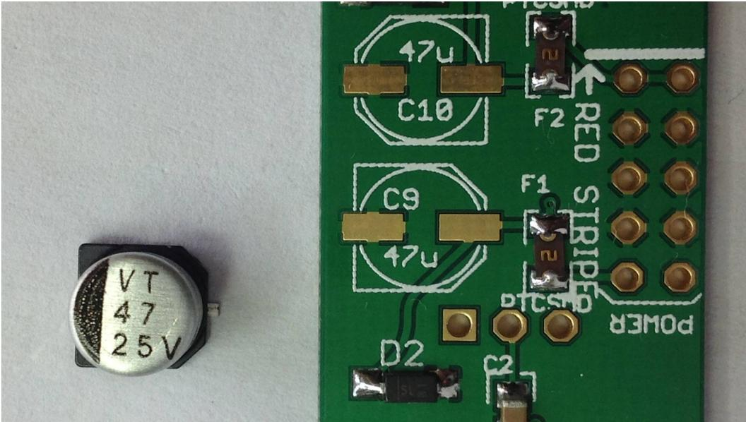
Again, remove one of the devices from the tape, offer it up to the PCB. Note how the pins sit on the pads. You'll probably notice there isn't a huge amount of room to get the soldering iron on the pad with the component on it. We have a technique for this.
