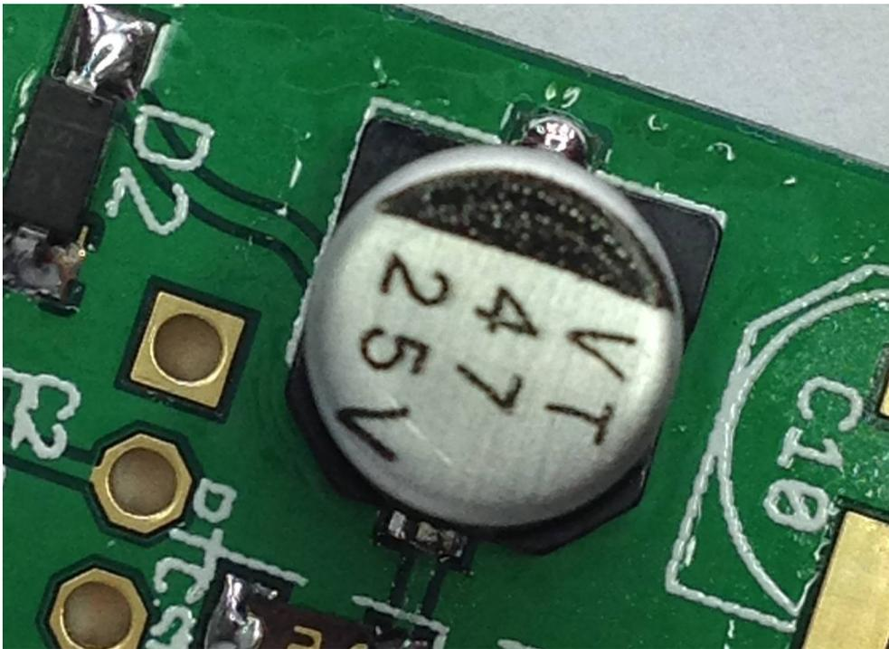
Once you've done that pad, go back to the first pad, apply some fresh flux if you're using it & add some more solder to the joint using a similar technique you just used on the second pin.
