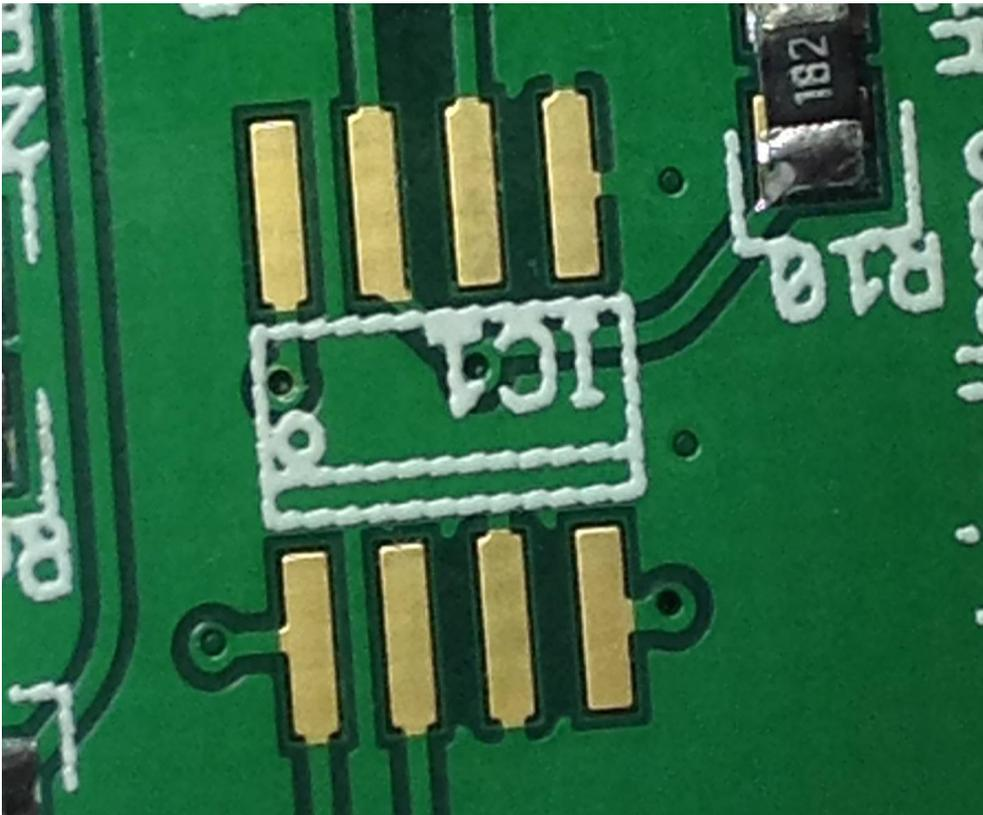
*Illustration 21: silk screen for IC1 showing the dot marking the location of pin 1, and the second line for devices that have a sloping face on the package*
