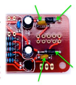
NOTE! Do not heat the diodes excessively or you will damage them, you should be aiming to solder quickly and neatly.
