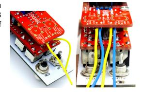
The wires shown in blue go from RTN\_RNG and SND\_RNG on the PCB to the grounding rings.
