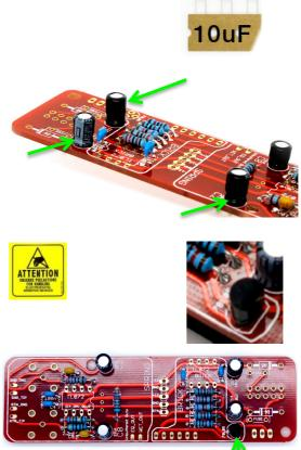
NOTE! Do not heat this part excessively or you will damage it, you should be aiming to solder quickly and neatly.
