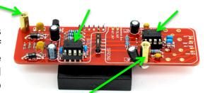
NOTE! This spacer may cause the C2 Electro Capacitor to lean over but this shouldn't cause a problem.
