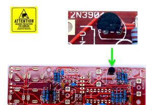
NOTE! Do not heat this part excessively or you will damage it, you should be aiming to solder quickly and neatly.
