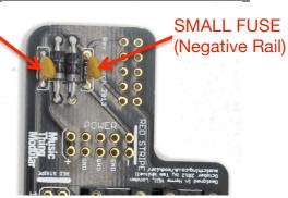
This image shows an older revision where both fuses were the same size. However all Backpack kits are now being issued with a new large fuse for the positive rail, this is required to run more than two expanders, e.g. when using PULSES, VOLTAGES and VACTROL MIX together. The smaller fuse doesn't need an upgrade. You can buy the fuse upgrade separately here:
