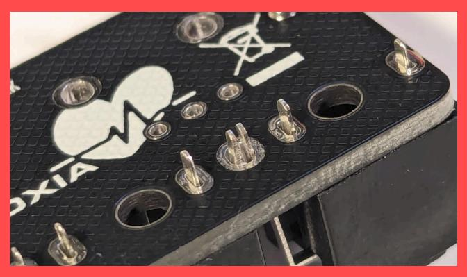
Finally, insert the potentiometers – you may have to bend the leads a bit to make it fit just so, and it may take a bit of pressure to go in, although it should not require violence. Verify that everything is inserted correctly before proceeding to solder the pins.
