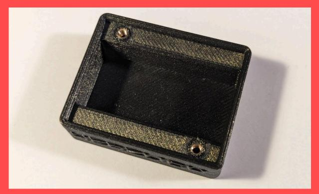
Repeat this process for both inserts, and finally place your module in the enclosure. The inserts will make it easy for the bolts to secure it in place. That's it, you're all done!
