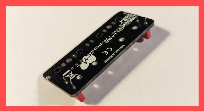
Next, install the 3,5mm jacks. Pay close attention here, as the jacks must be inserted so that they share ground pins (the exposed pin) in pairs. It is **very important** that you insert them like this before soldering, because it's going to be a real hot mess to sort out if you don't. You have been warned.
