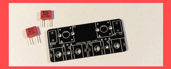
By bending the leads slightly once inserted, you should be able to turn the board around and solder the legs in place easily. Once they are soldered, turn the board over and verify that the capacitors are nice and flush against the board, before cutting the leads close to the board. If something isn't flush reheat the solder joint and press the errant capacitor flat against the board as you let the joint cool. This procedure is applicable to most electronics DIY, so keep it in mind as you go!
