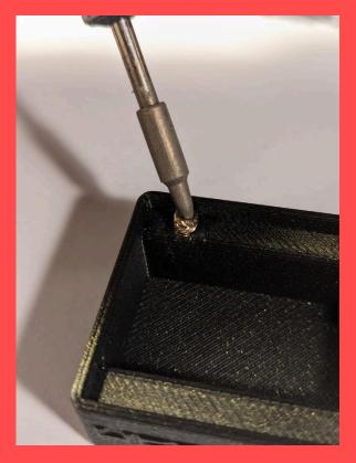
The heat from your soldering iron will disperse into the brass insert, which in turn melts the plastic. Do *not* use more than a slight amount of pressure, let the heat do the work – you're merely guiding the nut into the hole, not pressing it in. Once the nut is just below the surface, give your iron a little twist and release the nut. If you have done this correctly, the nut should stay in place as the plastic hardens around it, forming a very secure connection.
