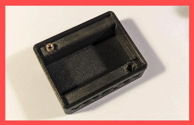
Using a hammer may seem tempting, but you have a much better tool at your disposal: your soldering iron. Place one of the nuts over the hole, so that the narrow end is pointing towards the hole. Now, heat your soldering iron to normal working temperature, and use the tip to gently press the insert into the plastic.
