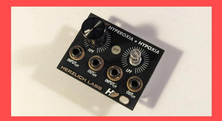
To test the device, simply patch in a harmonically rich signal (such as a square wave) in either the HPF or LPF input, and listen to either the HPF or LPF input to get HPF, BPF or LPF. If something is not working as expected, try reflowing your solder joints.
