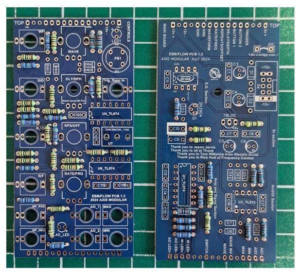
Begin your build by populating and soldering all the resistors. Although I've printed the values for you it's still wise to check each one with a multimeter before placing and soldering in its designated location on the PCB.
