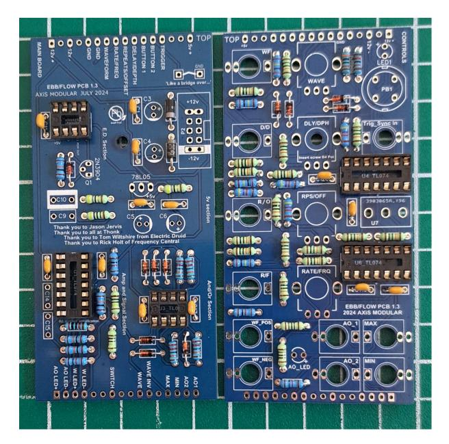
Locate the 11 100nf capacitors(labelled 104) and place at:
