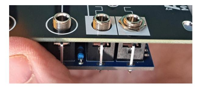
Once happy, solder all jack pins to the PCB. Then remove the panel.
