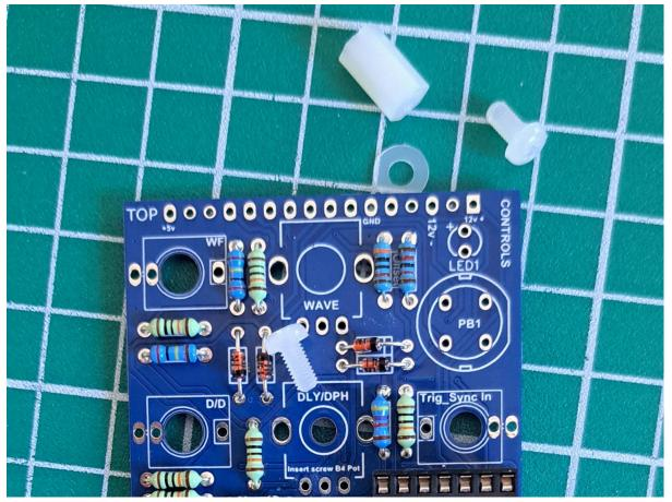
In the kit you'll find two nylon M3 screws, one spacer and a washer. It's important to fit this in part now as it will fix the PCB sandwich in place near the end of the build.
