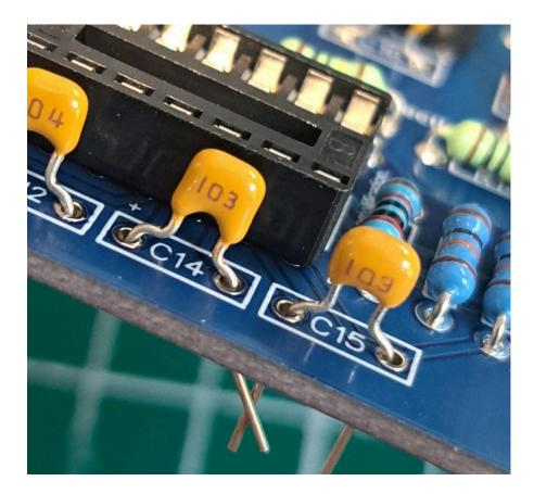
Next locate the two 10nf capacitors(labelled 103) and place it at:
