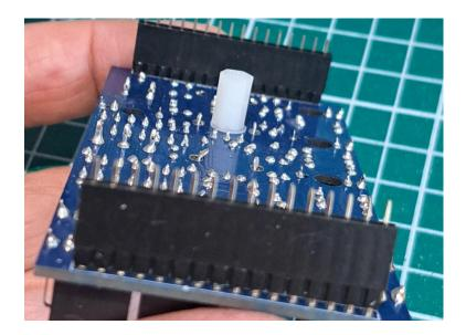
Then place the Main PCB onto the female headers. Make sure they are the correct way up as shown.
