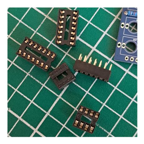
Place the 5 IC sockets into the PCBs, use either tape or bend a couple of corner legs to allow you to flip the PCB over to solder without them falling out.
