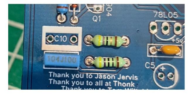
Next up you have one 100nf box capacitor(marked 104J100) Solder, trim, reflow if needed.
