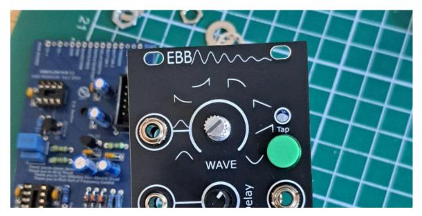
Use some tape to hold the button in place and make sure the LEDs are sitting into their holes on the panel, turn over and solder all the control parts you have just fitted. Take care and don't rush.
