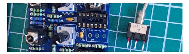
Place the switch where indicated on the PCB.
