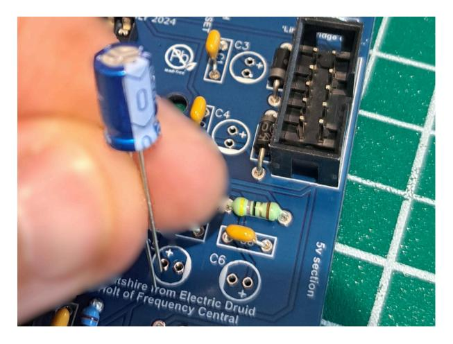
Find and place all four electrolytic capacitors. Make sure to orientate them correctly. The negative side is the striped side, positive is the longer leg.
