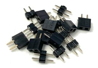
The sockets are placed on the back PCB on the same side as the SMD presoldered components. **Don't solder them yet!**
